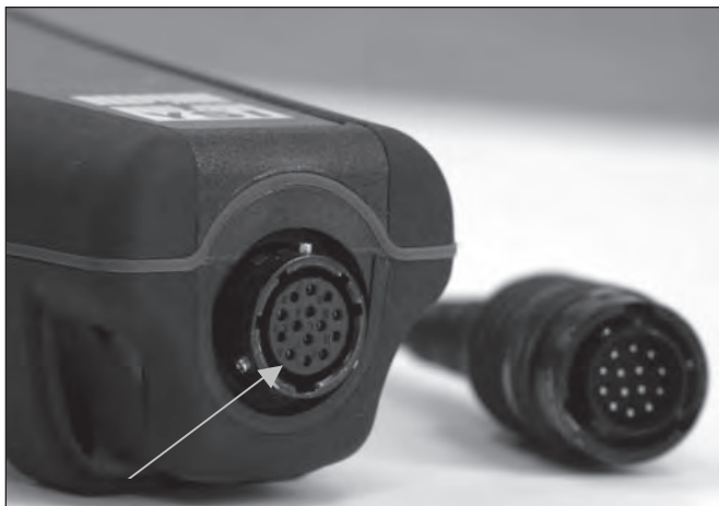
Figure 3, Note the keyed connector.
